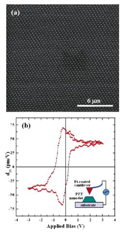
Figure 3. (a) SEM image of a large array of ferroelectric  $Pb(Zr_{0.40}Ti_{0.60})O_3$  (PZT) nanodots on a Nb-doped SrTiO<sub>3</sub> single-crystal substrate with (111)-orientation, together with (b) a typical piezoelectric hysteresis loop obtained from a single PZT nanodot. Schematic of a piezoresponse-scanning force microscopy (PFM) measurement is presented as an inset in (b).
