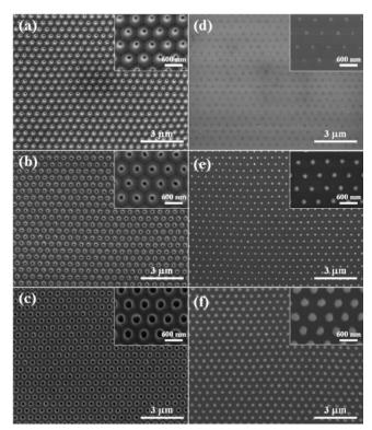
**Figure 2.** (a-c) SEM images of Au nanotube membranes fabricated from nanoporous AAO templates with different pore diameters (182, 222, and 326 nm for a, b, and c, respectively). Electrodeposition was carried out at a current density of 1.5 mA/cm<sup>2</sup> for 50 s at 17 °C. (d-f) SEM images of 2-D arrays of Pt nanodots sputtered on Si substrate by using respective membranes a-c. The high magnification views of each micrograph are presented as inset.
